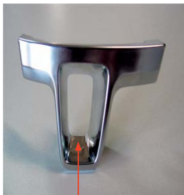
Abb. 5: Messpunkt zur Schichtdickenmessung Figure 5: Measurement point for deposit thickness measurement
